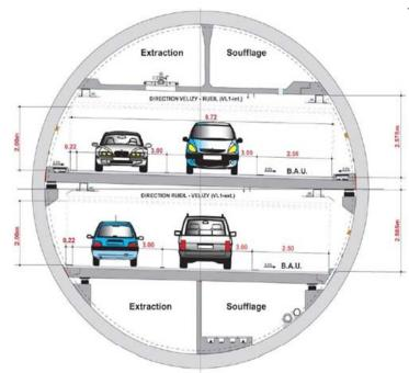
Tunneling has become substantially faster, simpler, more compact, more reliable and cheaper compared to the tunneling of H-3 Freeway. Recent tunnels in Paris and Miami have shown this. Only one tunnel is needed (see Figure). It provides two new lanes per direction in separate decks inside one bore.
